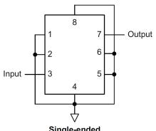
Single-ended Input and Output Filter Primary Connection Diagram
